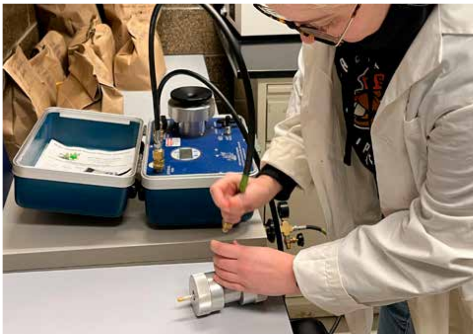
At the U.S. Department of Agriculture Agricultural Research Service (USDA-ARS) Horticultural Crops Research Lab in Corvallis, Oregon, scientists (above) use cavitation chambers to simulate drought stress in tree stems brought from the field. Below, scientists built an experimental plant hydraulics apparatus to measure the flow of water through a cut stem. The rate of flow can inform researchers about how well the plant can move water to support growth and metabolism. COURTESY OREGON STATE UNIVERSITY
