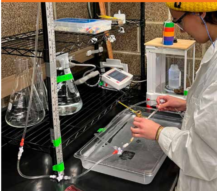
At the U.S. Department of Agriculture Agricultural Research Service (USDA-ARS) Horticultural Crops Research Lab in Corvallis, Oregon, scientists (above) use cavitation chambers to simulate drought stress in tree stems brought from the field. Below, scientists built an experimental plant hydraulics apparatus to measure the flow of water through a cut stem. The rate of flow can inform researchers about how well the plant can move water to support growth and metabolism. COURTESY OREGON STATE UNIVERSITY
