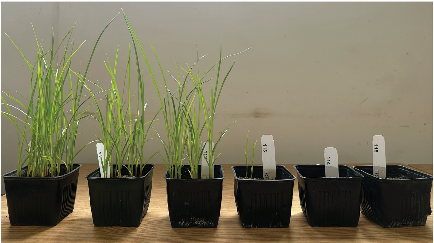
Yellow nutsedge plants 28 days after treatment with increasing rates of pulse electric field. PEF rates (L to R) were 0, 15, 30, 60, 125, and 250 J cm 3 .
