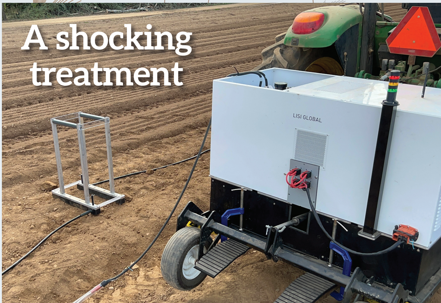
Overview of pulse electric field application in nursery beds near Boring, Oregon, in the fall of 2023. PHOTO COURTESY OREGON STATE UNIVERSITY
