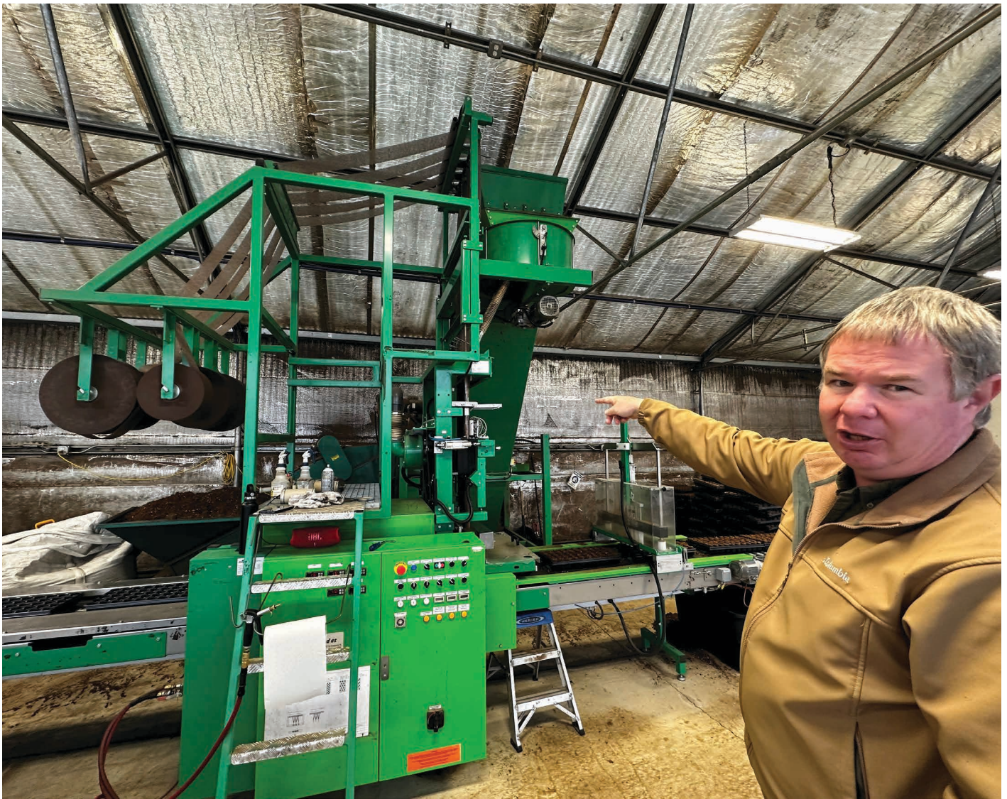
Customer Service and Shipping Manager Clayton Moore Jr. gives a tour of the Ellepot machines and explains how they work at North American Plants in McMinnville, Oregon. Rolls of biodegradable paper spool into the machine and the paper is shaped into a tube and the machine fills the tube with planting medium (above and below). Different papers are formulated to last different lengths of time, Moore said. PHOTOS BY VIC PANICHKUL
