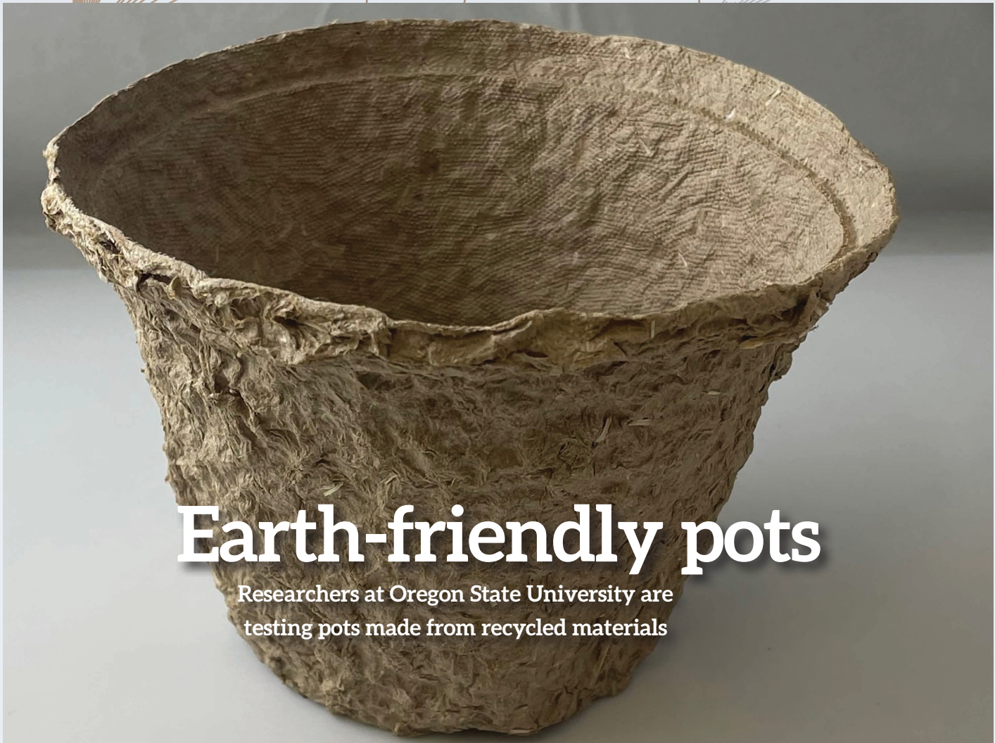
Nursery biopots made with recycled cardboard, hemp hurd, and apple pomace. PHOTO COURTESY OF OREGON STATE UNIVERSITY
