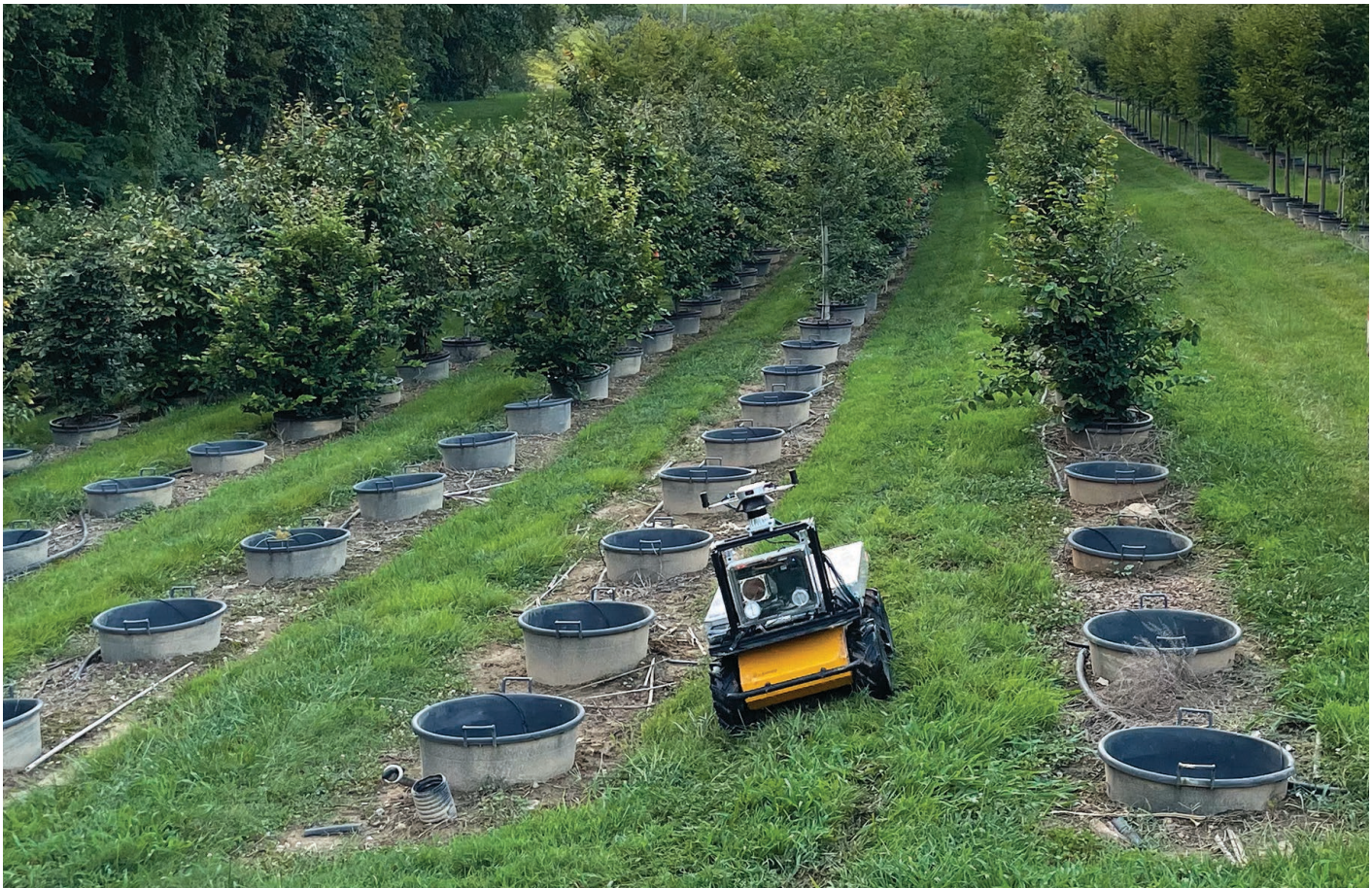
moss, a new robotics company, is developing an autonomous robot that can count plant inventory (above) and because it scans the entire plant in three dimensions, it can also extract the height of the trees and potentially the caliper as well (below). PHOTO COURTESY MOSS
