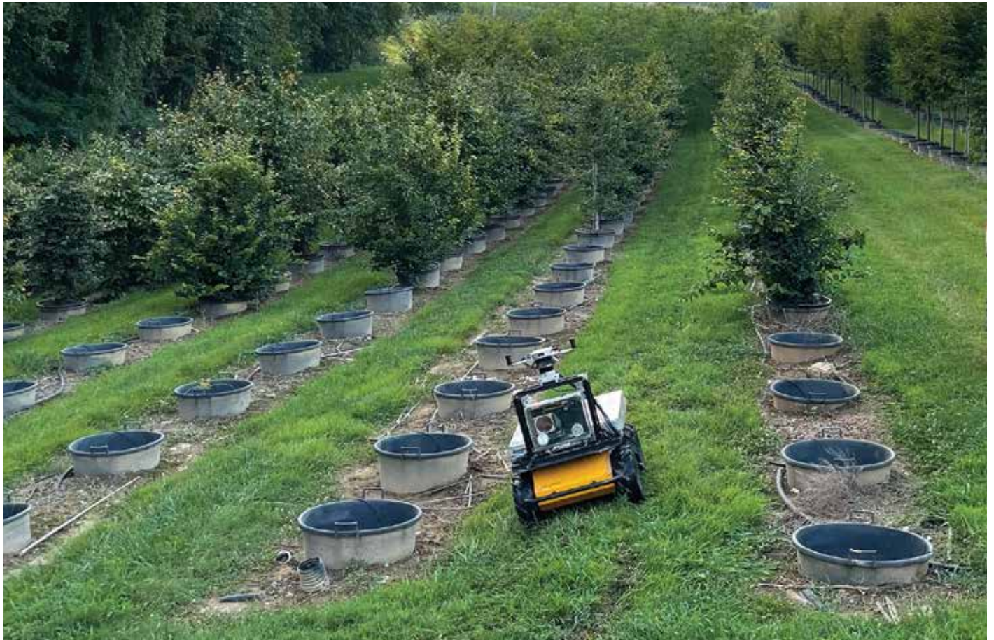
mos, a new robotics company, is developing an autonomous robot that can count plant inventory (above) and because it scans the entire plant in three dimensions, it can also extract the height of the trees and potentially the caliper as well (below). PHOTO COURTESY MOSS
