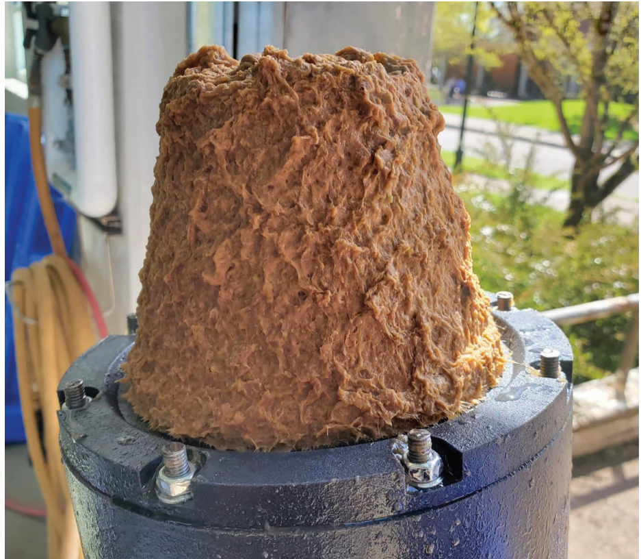
A 3D mold for creating nursery biopots. PHOTO COURTESY OREGON STATE UNIVERSITY
