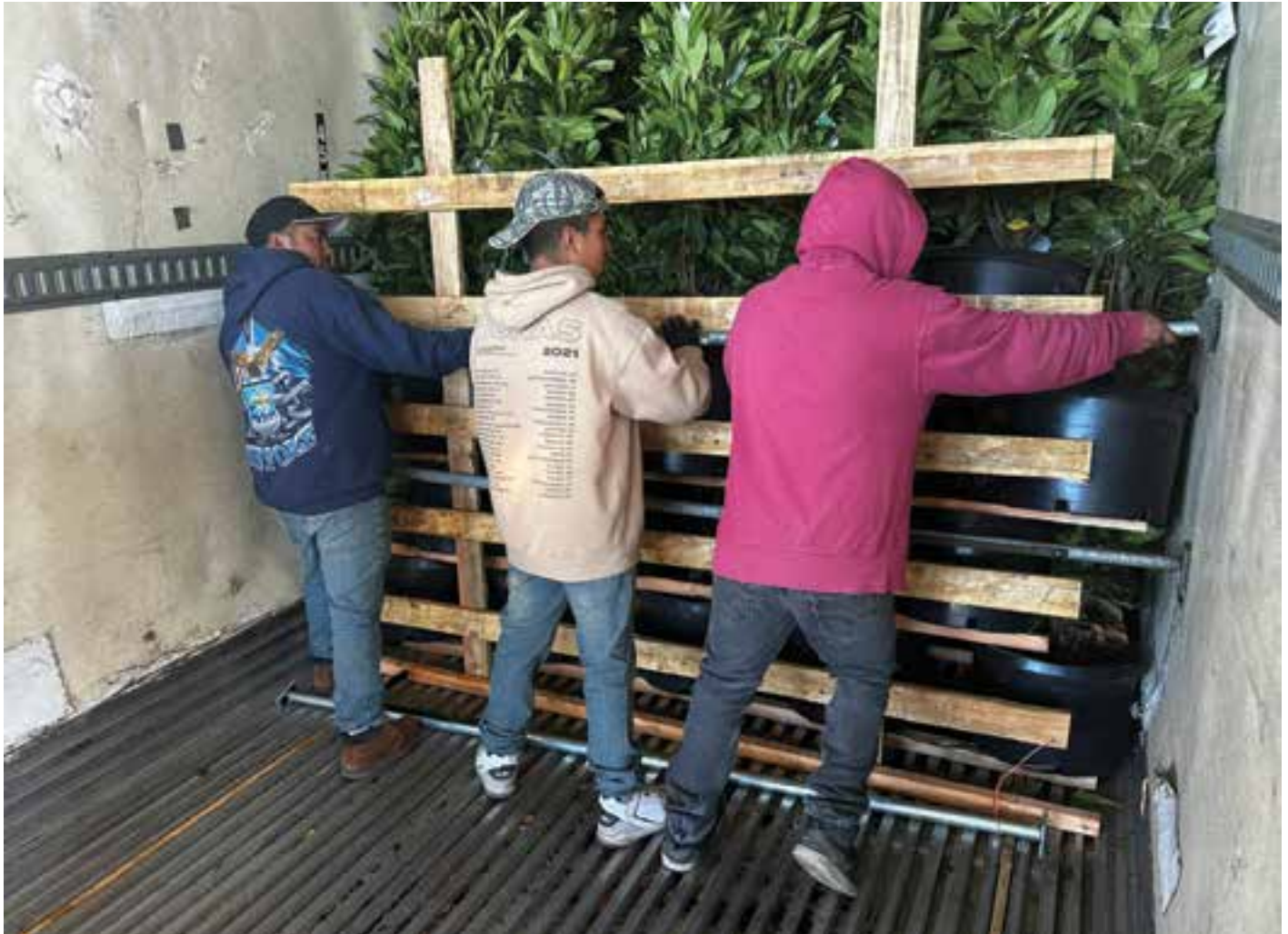
Workers add load separators and bracing to a shipment at Woodburn Nursery & Azaleas to keep the plant material from shifting during transit.
