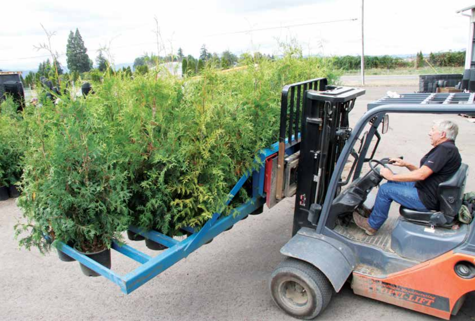
One of the hallmarks of Krueger's Tree Farm is the use of technology to save labor. Here, Dick Krueger drives a heavy-duty forklift from Wurdinger equipped with a special fork that allows for lifting of more pots. PHOTO BY VIC PANICHKUL
