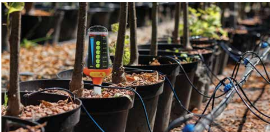
SAGE is a soil water monitoring tool developed by Stevens Water Monitoring Systems. PHOTO COURTESY OF STEVENS WATER MONITORING SYSTEMS
