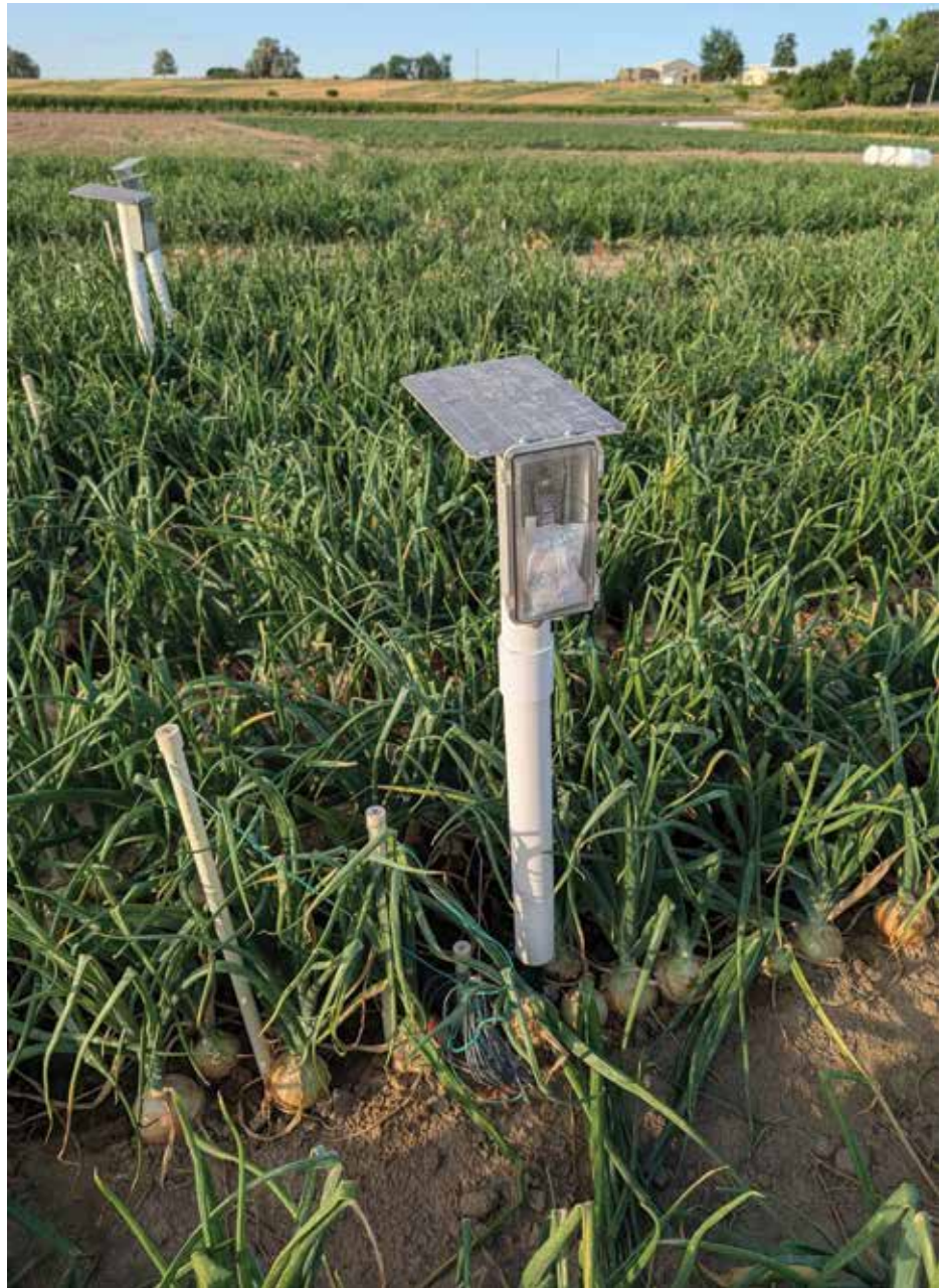
Researchers at Oregon State University are building and testing an affordable soil moisture monitoring system that utilizes open-source electronics. PHOTO COURTESY OF OREGON STATE UNIVERSITY
