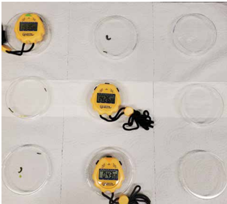
Figure 4. Host range testing arenas (each row is a replicate). In no-choice trials, Eriborus sp. individuals are moved across each row to sequentially encounter box tree moth, non-target, box tree moth. Each encounter lasts 30 min or until attack occurs. PHOTO COURTESY OF USDA-APHIS
