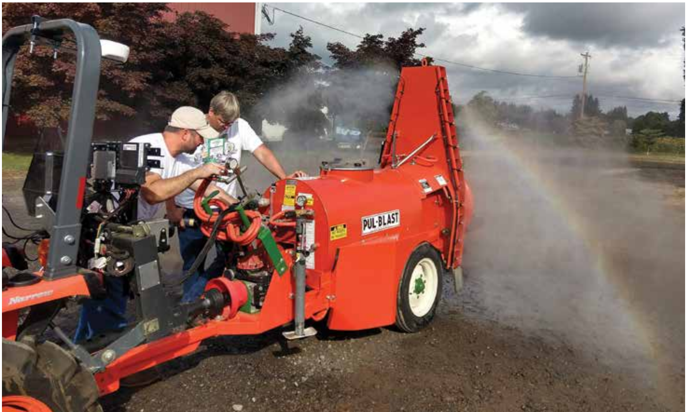
USDA-ARS researchers fine-tune a newer generation of the Intelligent Sprayer System, retrofitted onto a conventional air-blast sprayer. The retrofit uses LiDAR technology to detect plant canopies and control individual nozzles, adjusting spray applications as the sprayer moves through the crop. PHOTO COURTESY OF OREGON STATE UNIVERSITY
