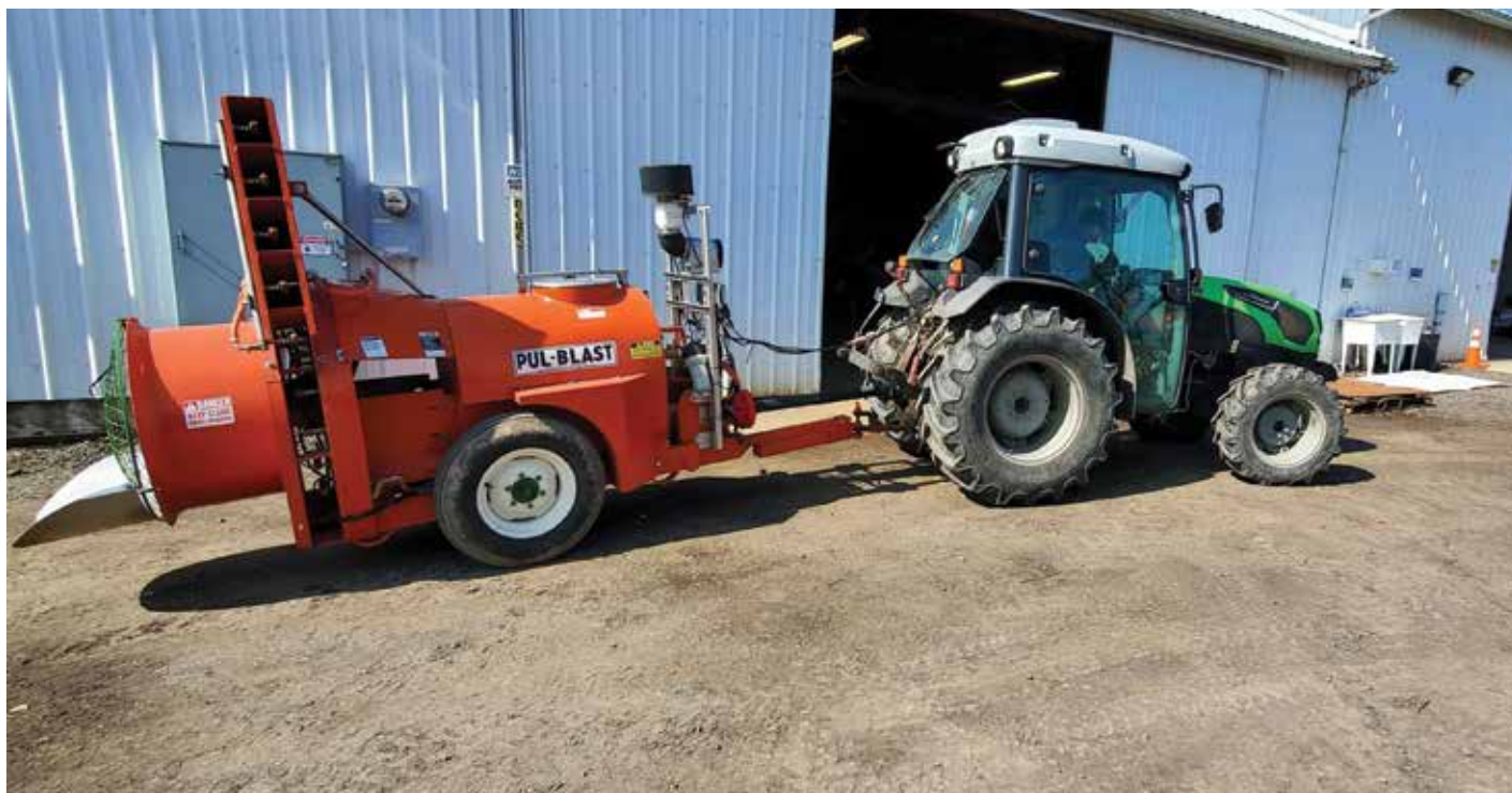
The Red Robin, one of two Intelligent Sprayer research platforms developed and operated by Oregon State University, during field trials at a commercial Oregon nursery. Long-term partnerships with growers have been instrumental in moving intelligent spraying from experimental prototypes to practical commercial adoption. PHOTO COURTESY OF OREGON STATE UNIVERSITY
