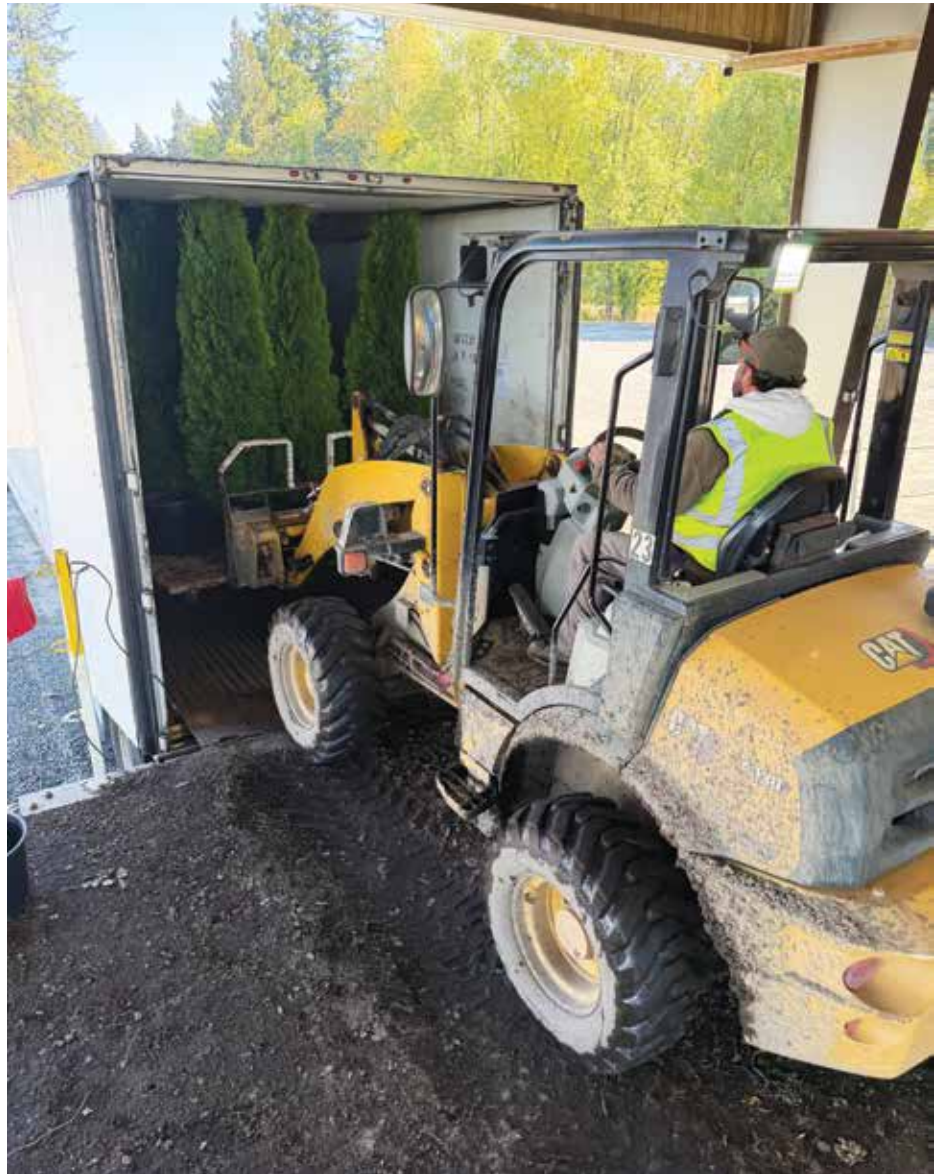
Crew Leader Celso Barron drives an articulated loader to carry a pallet of arborvitae into a truck at Bountiful Farms. For safety and efficiency, Bountiful Farms uses well-lit articulated loaders to load trucks and assigns a crew leader for each load to supervise loading. PHOTO BY VIC PANICHKUL
